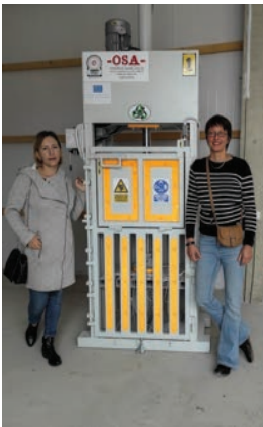
Zero Waste Montenegro staff in front of the Hydraulic Press (Pressure force: F=120kN (12 tons), Manual hydraulic controls)
